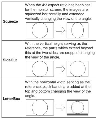
• When output is selected for the color bar, the mode is fixed to Squeeze.
